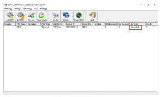
Note: If the "Net State" column displays a failed connection, please check whether the TCP module and the current PC are in the same network.
