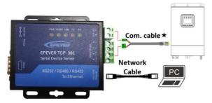
After the TCP module is successfully connected to the PC (the Link indicator is green ON), set the IP address of the computer and TCP module in the same network segment.
