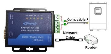
★ Select an appropriate communication cable per the communication interface of the controller, inverter, or inverter/charger.
