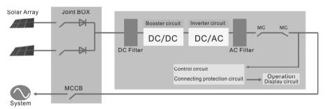
Figure 2: Main Circuit of KSG-10K/12K/15K/17K/20K Inverter
