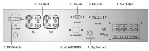
Figure 3: Interface of KSG-10K/12K/15K/17K/20K Inverter
