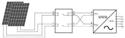
side of inverter via two groups of parallel input terminals.
