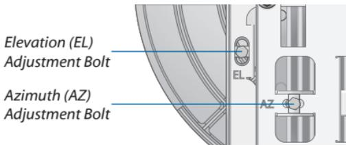
3. **Master** Aim the *Master* at the *Slave*. If necessary, adjust the *Master's* position on the pole:
