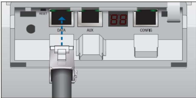
3. Create a strain relief for the Ethernet cable by feeding a cable tie through the tie slot under the cable. Then wrap the cable tie around the cable and tighten.
