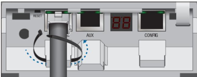
4. Connect the other end of the Ethernet cable from the *DATA* port to the Ethernet port labeled **POE** on the PoE Adapter.
