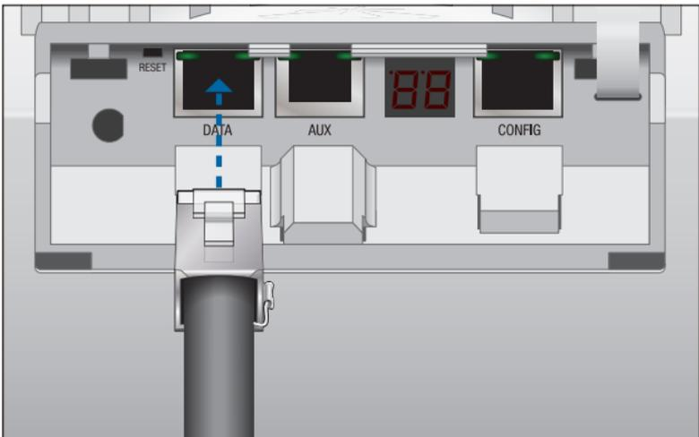
3. Connect the other end of the Ethernet cable from the *DATA* port to the Ethernet port labeled **POE** on the PoE Adapter.
