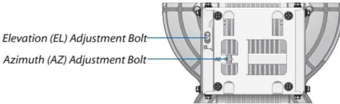
6. **Slave** Aim the *Slave* at the *Master* to achieve the strongest received signal level on the *Slave*'s numeric LED Display, which is located next to the *CONFIG* port. If necessary, adjust the *Slave*'s position on the pole:
