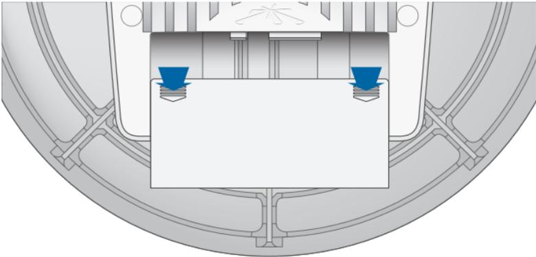
2. Connect a TOUGH Cable or other outdoor, shielded CAT5e/6 cable to the *DATA* port.
