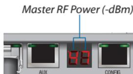
2. **Master** Adjust the azimuth and elevation of the *Master* until the other installer sees the strongest received signal level displayed on the LED Display of the *Slave*.
