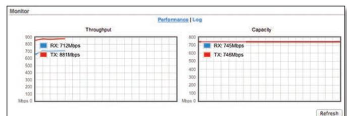
*Throughput* displays the current data traffic on the *DATA* port in both graphical and numerical form. The chart scale and throughput dimension (Bps, Kbps, Mbps) change dynamically depending on the mean throughput value. The statistics are updated automatically.
