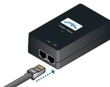
5. Connect an Ethernet cable from your network to the Ethernet port labeled **LAN** on the PoE Adapter.
