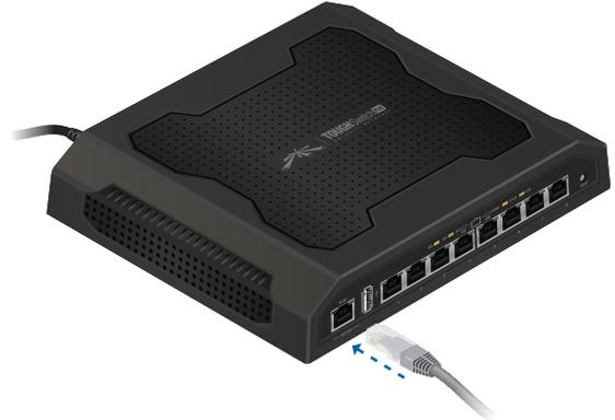
2. Connect Ethernet cables from the Ethernet ports of your devices to the numbered ports of the TOUGHSwitch.
