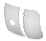
b. Slide the Side Reflector Panel down until the top edges of the panels align. The Side Reflector Panel is captured when both heads of the mounting studs are positioned over the narrow opening of the slotted holes.
