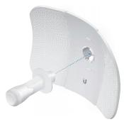
6. Press both sides of the *Port Cover* and detach it from the *Feed Receiver*.
