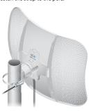
11. Loosen the lock nut on the *Ball Joint Mount*, and aim at the other end of the wireless link. Use the bubble level to ensure level alignment, and then lock the aim by hand-tightening the lock nut.
