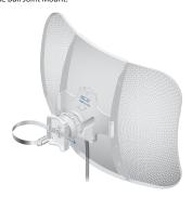
10. Wrap the Metal Strap around the pole. Use a 7 mm socket wrench or screwdriver to turn the screw clockwise and securely fasten the strap to the pole.
